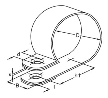
$\begin{array}{ll} d & = 8.4 \\ \text{Diameter D} = 50 \\ \text{h1} & = 37.5 \\ \text{I} & = 8.5 \\ \text{s} & = 1.0 \\ \text{Width B} & = 20 \\ \end{array}$
